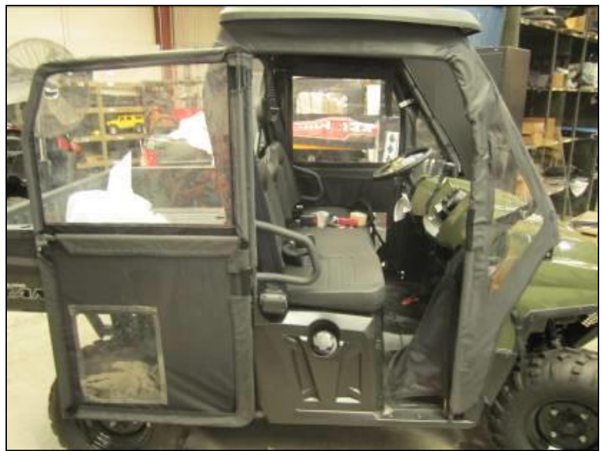
14. Mount the doors by guiding the pins in the back of the door frame onto the hinge barrels along the Rear Hangar Bar.
